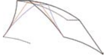
Distortion of the flank with form relieved thread milling cutters with varying rake angles
